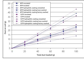
Figure 4. Effect of Fin Density, Coatings and Coil Cleanness on Dust Accumulation
