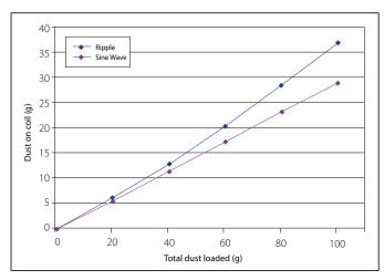
Figure 5. Effect of Fin Pattern on Dust Accumulation
