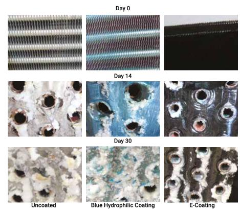
Figure 2. Salt Spray Test Samples and Results
