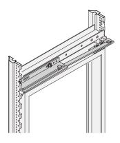
Swing frame stop kit for 19" swing frame (max. swing angle 120° or 160°).
