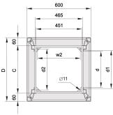
Fixed spacing between front and rear 19" plane.
