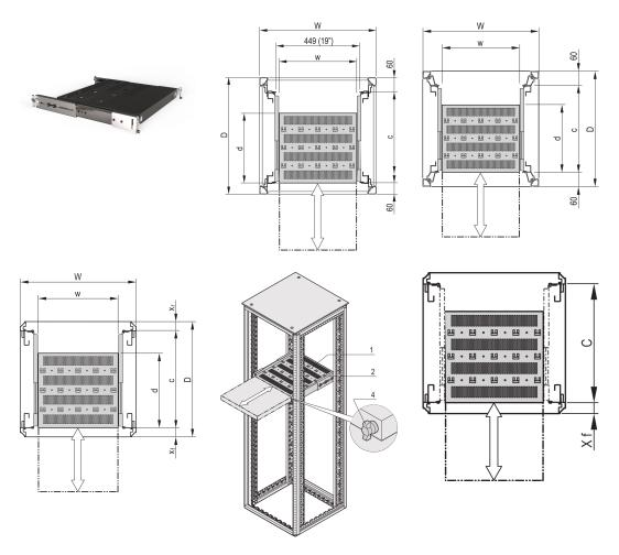
Varistar, Novastar and Eurorack 19" Shelf, Stationary with 70 kg load capacity, perforated for ease of assembly.
