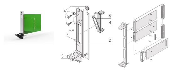
The FMC bezel are in accordance with Vita 57.1 specification. Covers the cut out in the overall front panel.
