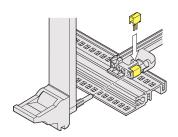
Based on the IEEE standard guide rails and handles can be coded to avoid the insertion of a wrong board into the wrong slot.
