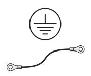
Cables carrying high voltage current may effect other cables in the bundle and hence electronics in the rack. The earting of the cable channel ensures that such mishaps are protected.
