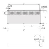
The perforated rear panel, Al, 2.5 mm is unshielded. The rear side is conductive.
