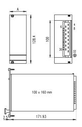
Front Panel for nVent SCHROFF 19" compatible Power Supply. Flat front panel with vertical grooves for stainless steel EMC Contact Strips.
