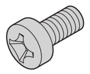
Pan head screws are a common head type of non-countersunk screw head used in self-tapping screws, self-drilling screws, and machine screws. They have wide heads, a flat bearing surface, high vertical, chamfered, or curved sides, and a flat or slightly domed top surface with a recessed socket.
