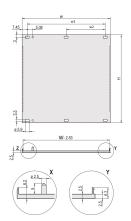
U-profile front panel for textile EMC gasket.
