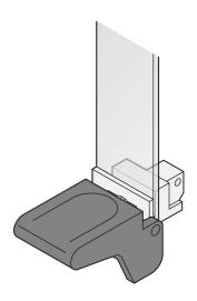
Extractor handle key form 1, can be used to extract PCBs. The handles are available in black or grey and top and bottom versions.
