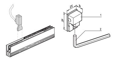
power connector for busbar achieves internal power distribution designed to reduce server complexity and providing a separable connection that ease assembly, inspection, and troubleshooting.
