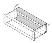
The rear hood is used as a shielded rear boundary and requires 60 mm space. Therefore if the rear hood is used, the side panel depth must be 60 mm greater than the board depth. Contact between the rear hood and the horizontal rails is established by the stainless steel contact strip for the cover plate. Thus no additional EMC sealing is necessary. Rear hood cannot be used simultaneously with rear corner profile.
