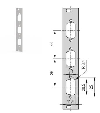
19" Front Panel with SUB-D Cut-Out or FDDI Cut-Out.
