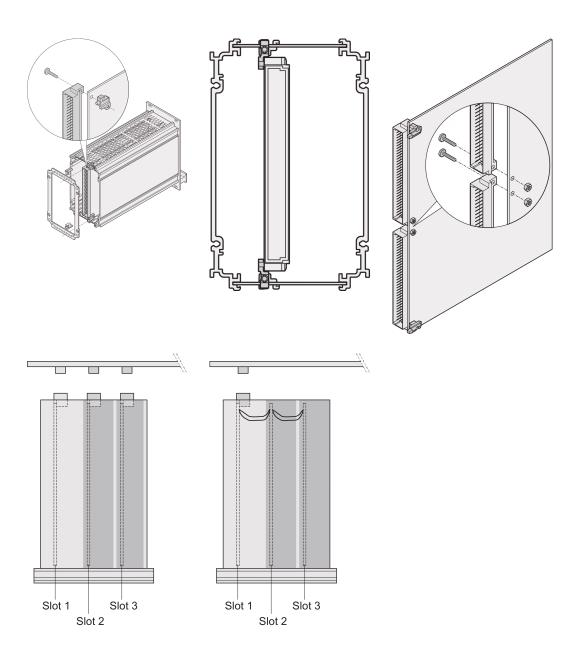
PCB is inserted into the guide groove of the left side Panel or that of the side Panel rear angle, From Slot 2 on.
