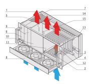
4 U CompactPCI System with vertical Card Cage for eight 3U Boards, eight RTM Boards and one 3U Pluggable Power Supply.
