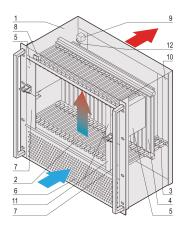
10 U CompactPCI System with PSB for fourteen 6 U Boards, fourteen RTM Boards and up to four 3U pluggable Power Supplies.
