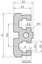
The assembly kit includes a center rail and 2 adapters plus assembly material. The kit enables use in a 6 U CompacPRO, and splits the case into  $2 \times 3$  U sections.
