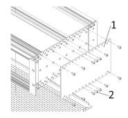
Aluminium Side panel 3mm to increase the EMC shielding effect of the subrack by covering the not needed cut-outs.
