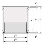
Telescopic slides with guiding profile for fitting in cabinets with 25 kg load capacity.
