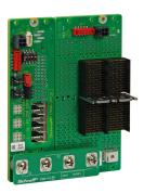
Power Backplane for CompactPCI Serial applications. Up to 4 Power backplanes can be connected to increase power or for redundancy.
