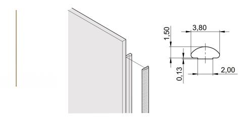
The textile EMC gaskets are inserted into a slot on the right hand side of the U-shaped front panels. The gaskets are glued to the front panel.
