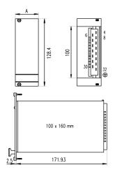
Front Panel for nVent SCHROFF 19" compatible Power Supply. Flat front panel with vertical grooves for stainless steel EMC Contact Strips.
