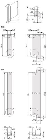
Plug-in unit, with IEL inserter/extractor black handle, 6 U, front assembly. The U-shaped front panel enable shielding with a textile gasket.
