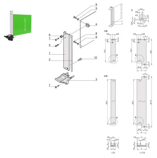
Plug-in unit, with IEL inserter/extractor black handle, 3 U, front assembly. The U-shaped front panel enable shielding with a textile gasket.
