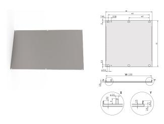
U-profile front panel for textile EMC gasket.
