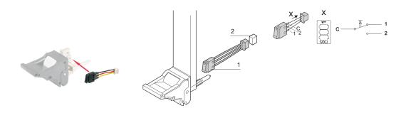
Micro Switch for IEL or IET handle. The micro switch fits also for the Offset versions of the handle.
