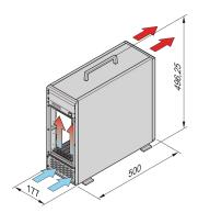
VME64 tower system for 7 VME64x boards 6 U, 160 mm. The power for the system is supplied by a open frame power supply. A fan control module monitors the fans, the temperature and voltage.
