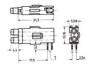
Double test sockets for mounting plane 1 and 2, short and long type.
