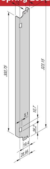
AdvancedTCA front panel for spring-loaded IEA handle with die-cast end piece.
