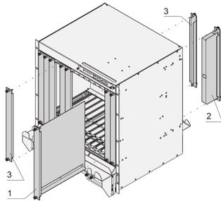
Advanced TCA front panels cover empty slots in a system. The additional air baffle blocks and guide the air in the right direction.
