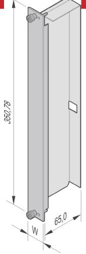
AdvancedTCA Air Deflector Filler Panel, Rear. Blocks the air in unused slots.
