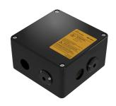
nVent Raychem JBU-100-A, JBU-100-A6 and JBU-100-L-A are modular junction boxes. The junction box can be installed on the pipe using a mounting bracket such as UMB or off-pipe using other means. The heating cable is typically brought into the box using the flexible conduit and C75-100-A gland kit. The junction box consists of terminal blocks to make the connections and four 3/4" through holes.
