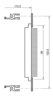
Perforated flat rail for connector mounting i.a.w. EN 60603-2 and DIN 41612, on VT horizontal rails.
