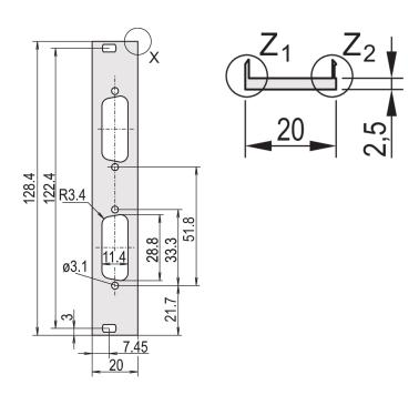
U-profile front panel with cutout for D-Sub connectors. Shieldable for textile EMC gasket.
