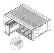
Additional securing of the rugged cover plate to protect against shock and vibration. The Kit will be screwed onto the top / bottom cover. A movable bolt engages under the horizontal rails and thus provides additional fixing.
