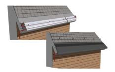
nVent RAYCHEM Roof Ice Melt (RIM) System is our premiere offering for roof & gutter de-icing in light to heavy snow load areas. The system consists of metallic panels that embed self-regulating heat tracing cable to provide high power output and an aesthetically pleasing roof de-icing solution. The RIM system includes panels specifically designed for eaves, valleys, channels, rakes and flat roof sections.
