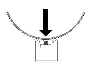
2. Rotate shield so it is positioned perpendicular to channel.
