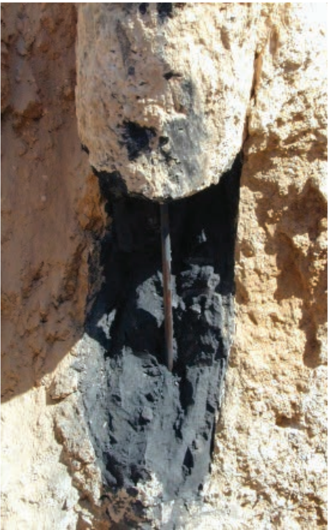
Figure 10: An exhumed ground rod in ground enhancement material
