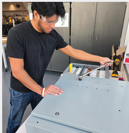
In preparation for push buttons and indicator lights, the students drill holes on the front door.
