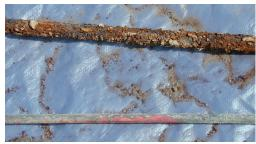
Top ground rod is galvanized steel, 3/4" x 10'. Bottom ground rod is copper-bonded, %" x 8'. Both ground rods were driven into the soil vertically at the Pecos testing site in Las Vegas, NV in December of 1992. Both ground rods were exhumed from the site in April of 2004. The loss of zinc on the galvanized steel rod resulted in excessive corrosion of the steel. The copper-bonded steel ground rods showed minimal corrosion.
