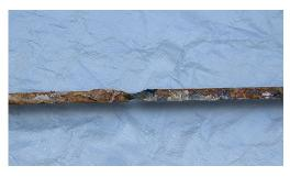
This is a galvanized steel ground rod driven into the ground vertically at the Pawnee testing site in Las Vegas, NV. This ground rod was buried from May of 1992 until March of 2003. The loss of zinc resulted in excessive corrosion of the steel. One area is reduced from a 34" diameter to approximately a 14" diameter due to the corrosion. The eventual failure would result in a potentially catastrophic
