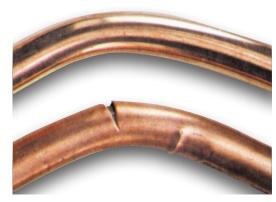
When an nVent ERICO brand of copper-bonded ground rod (top) and a copperclad rod are subjected to the same pressure load, the inferior copper-clad rod (bottom) develops cracks and creases to the outer sheath. Damage to the rod negatively affects its serviceable life and puts the integrity of the entire electrode
