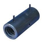
The side fill horizontal T-Series sleeve has vent holes located 90 degrees from the tap hole to facilitate side fill installations when the interferences of the structure will not allow top filling. Vent holes are added to horizontal sleeves to reduce air entrapment and help ensure proper filling of the sleeve.
