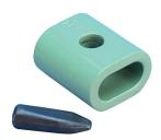
The nVent LENTON Quick Wedge splice consists of an ovalshaped steel sleeve and a wedge pin. The sleeve is positioned around two very short overlapping steel bars. The wedge pin is inserted into a handheld hydraulic pindriver and positioned on the sleeve. The pin is then driven through the pre-drilled hole in the sleeve and between the bars to complete the connection.
