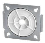
The nVent LENTON Interlok Form Saver Seal provides an easy and efficient means for securing nVent LENTON Interlok Grout-Fill Coupler variants to formwork. Designed for cast-in-place applications, simply click and tap the Form Saver Seal into the coupler and utilize the sturdy mounting plate to fasten onto the formwork. The integrated seal allows the secondary rebar to be inserted into the coupler and prevents concrete paste contamination and grout leakage out of the cavity.
