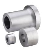
The DT16 head area exceeds 5x bar area (net 4x). The system is designed to meet Caltrans Ultimate performance with A706 grade 60 rebar, ASTM A970 Classes A, HA, and B performance with A706 and A615 grade 60 and grade 80 rebar.
