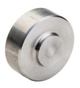
The nVent LENTON DR16 Ultimate Terminator is designed to eliminate reinforcing bar hooks and simplify bar placement. The Terminator head area exceeds 5x bar area (net 4x) and maintains greater design flexibility than hooked bars. The system is designed to meet Caltrans Ultimate performance with A706 grade 60 rebar, ASTM A970 Classes A, HA, and B performance with A706 and A615 grade 60 and grade 80 rebar.
