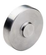
The nVent LENTON DR14 Ultimate Terminator is designed to eliminate reinforcing bar hooks and simplify bar placement. The Terminator head area exceeds 10x bar area (net 9x) and maintains greater design flexibility than hooked bars. The system is designed to meet Caltrans Ultimate performance with A706 grade 60 rebar, ASTM A970 Classes A, HA, and B performance with A706 and A615 grade 60 and grade 80 rebar.
