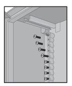
Self-Tapping Screws are Hi-Lo  $1/4-15 \times .88$ . They mount panels and accessories to DIN bosses on back of enclosure.
