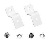
Designed to provide a simple and versatile method of mounting terminal straps. The Z-shaped brackets are 1.50-in. (38-mm) high. Brackets can be attached to panels or to enclosure walls. A terminal strap is then installed on the brackets. Terminal straps must be ordered separately. Spacing between brackets will depend on the number and size of terminal blocks installed on the terminal strap. We recommend a maximum spacing of 15 in. (381 mm) for an average installation.
